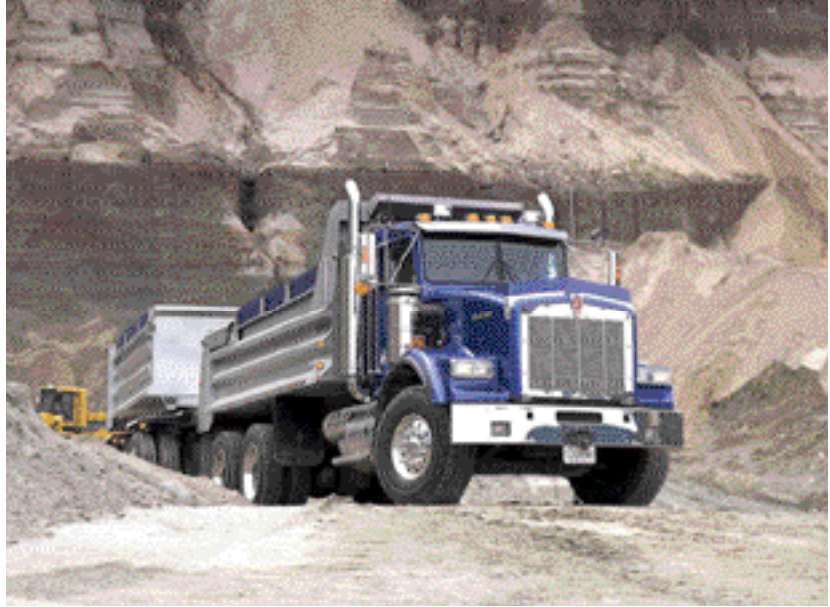
Frame rails usually need to be reinforced for hauling heavy loads.
